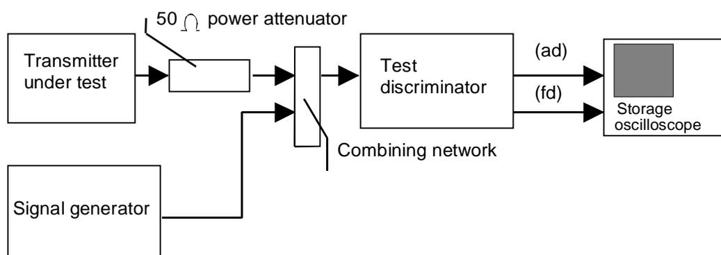
**Figure 3: Measurement arrangement**
